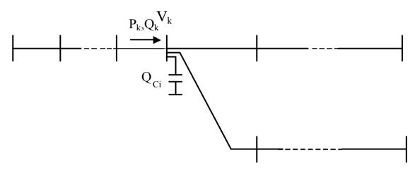
$$l_{k} = r_{k}(i_{Pk}^{2}) + r_{k}(i_{Qk}^{2}) = r_{k} \left( \frac{P_{k}^{2} + (Q_{k} - Q_{ci})^{2}}{V_{k}^{2}} \right)$$
