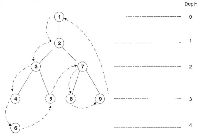
The backward DP procedure traverses the network with paths inverse to preorder. In this example: 9-8-7-5-6-4-3-2-1
