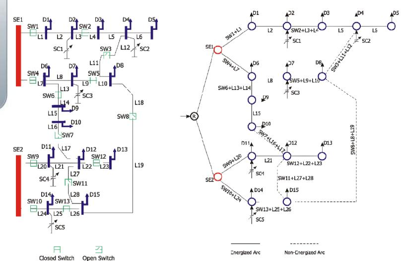
In most of cases it operates with a radial configuration
